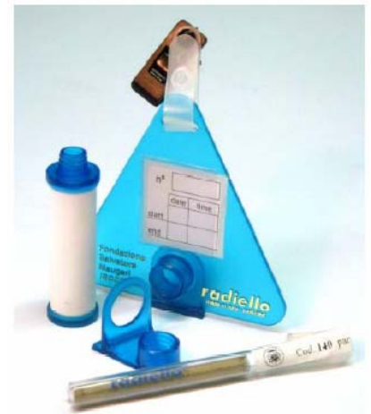
Pictured above: Radiello System - Diffusive Body, Supporting Plate, Adapter and Collection Cartridge in the Sealed Glass Tube.
